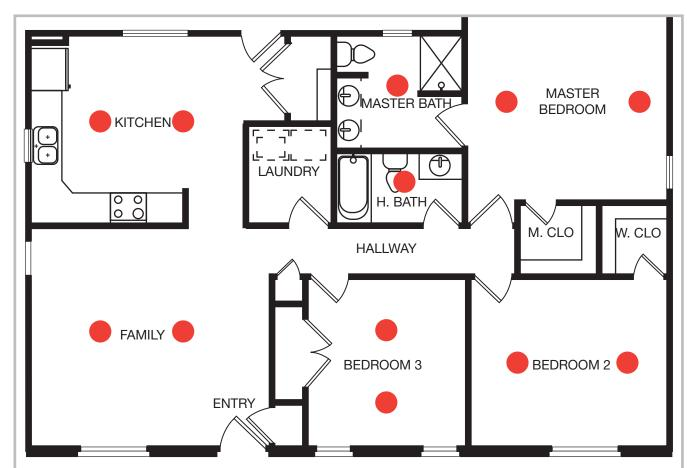
Connect 8 speakers to MTX and 4 speakers to SC4-100. Select source and control from a Nice Home Management panel or remote control.
