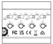
Ch 1&2 – Subwoofer – 20Hz Ch 3 – Speakers – 100 Hz Ch 4 - Speakers – 100Hz
