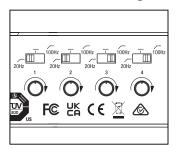
Ch 1 & 2 – Subwoofer – 20Hz Ch 3 – Speakers – 100 Hz Ch 4 – Speakers – 100Hz
